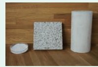
After hardening Left: Calcium carbonate powder Middle: Example of processing stone-like building materials Right: Test sample (Compressive strength 20 to 45 N/mm 2 )
